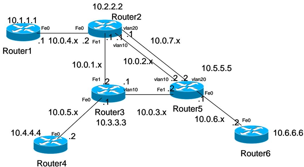
*IPv6 lab – Topology diagram & IPv4 addressing plan*
